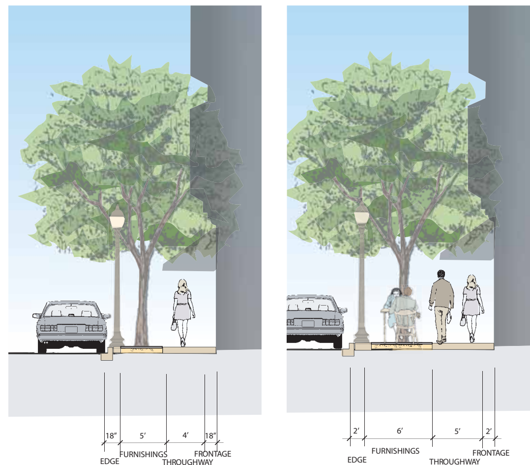
Figure 4.6 STANDARD MINIMUM (LEFT) AND RECOMMENDED (RIGHT) SIDEWALK WIDTHS, USING NEIGHBORHOOD COMMERCIAL STREETS AS AN EXAMPLE
