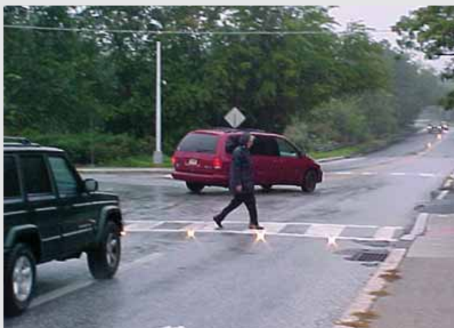
In-roadway flashing lights are a relatively new device to help enhance crosswalk visibility
