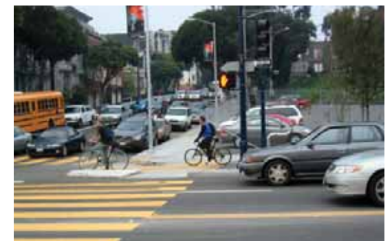
Placing parking on the median side of the local access lane can improve connection between the sidewalk and the local lane, and better buffer the sidewalk and shared area from the higher-volume thruway lanes.
