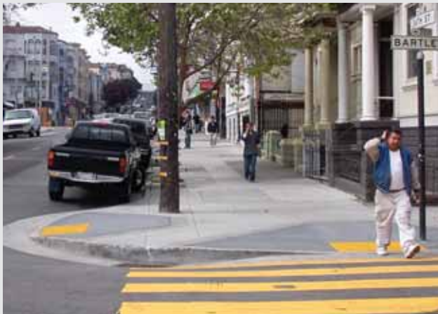
▲ Accessible curb ramps should be provided at all corners, one per each crosswalk end.
