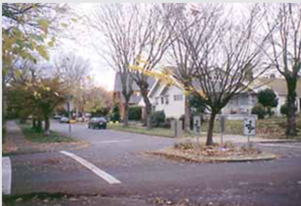
Traffic circles should include landscaping, including trees, and permeable surface. They may be designed to infiltrate stormwater runoff from the roadway.
