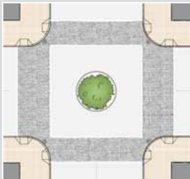
Traffic circles slow traffic in residential neighborhoods and provide added space for landscaping and stormwater infiltration.
