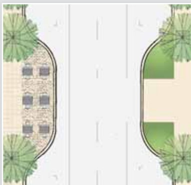
Top and Bottom: Curb extensions can create a variety of types of usable and attractive spaces for pedestrians at mid-block locations.
