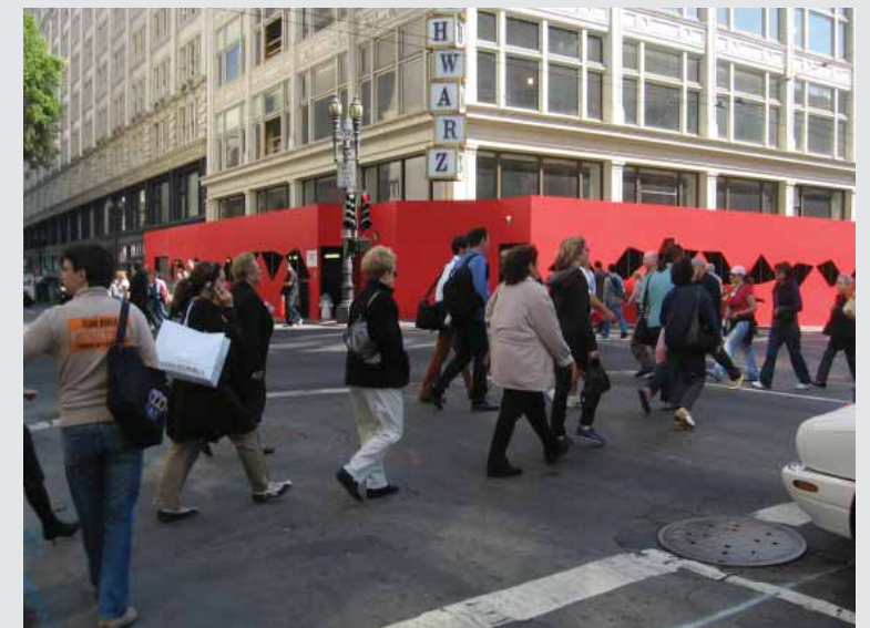
Pedestrian scrambles allow a dedicated signal phase for pedestrians to cross in any direction at an intersection
