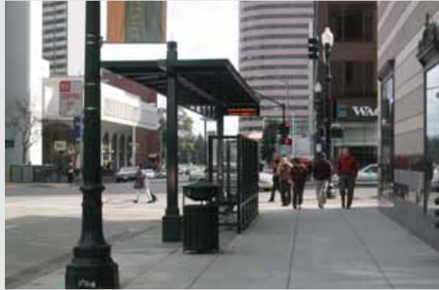
Curb extensions provide more space for amenities, passenger waiting, and sidewalk through travel at transit stops.
