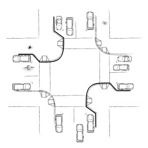
Where turning radii limit bulb-out dimensions, consider two bulb-outs at opposite corners, thereby shortening all crosswalk lengths
