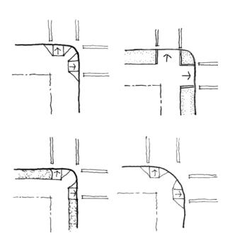
Accessible curb ramps should be provided at all corners, one per crosswalk end
