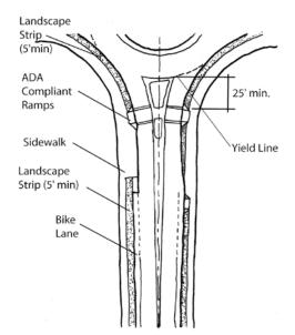
Roundabouts should be landscaped. Plantings should be less than 3- feet tall within 4 feet of the edge of the curb
