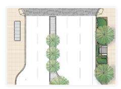
Medians provide space for trees and planting, visually break down the scale of the right-of-way, and create space for pedestrian refuges.
