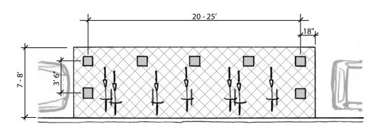
▲ Layout of an on-street bicycle parking space (typical). On-street bicycle parking should be designed with racks perpendicular to the curb, and elements to protect bicycles and racks from errant drivers.
