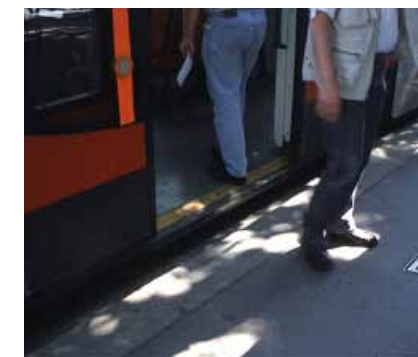
Ensure easy access for all passengers by entering directly from street level. Vienna, Austria
