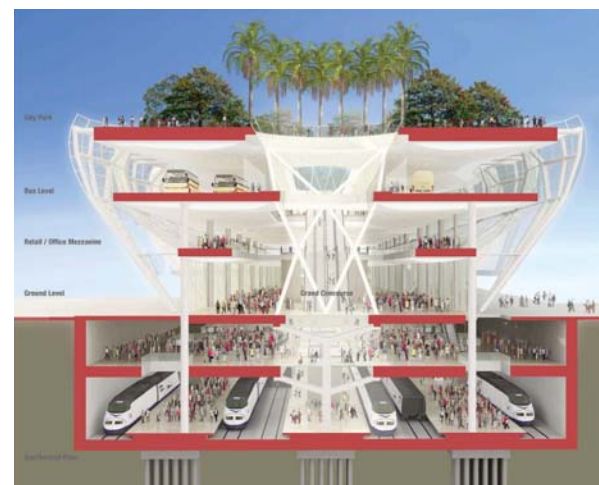
A cross section of the proposed Transit Center (Source: Pelli Clarke Pelli Architects)
