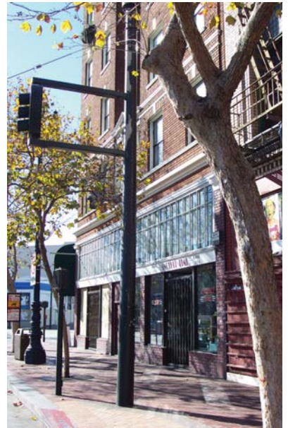
Building walls should be provided with articulation and interesting fenestration, such as the clerestory and recessed windows shown above.
