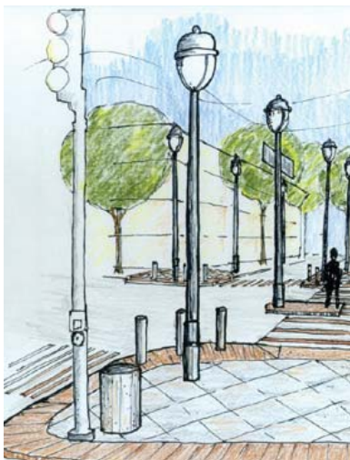
Lighting fixtures should be cut off or shielded to prevent upward light spill.
