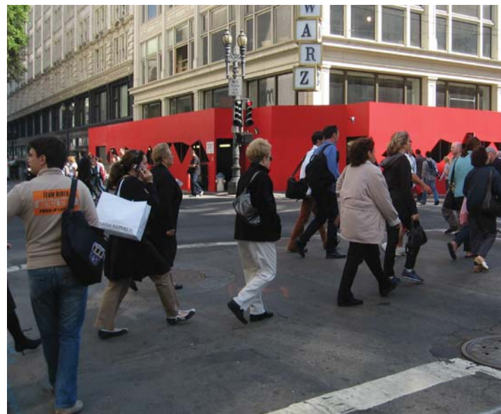
◀ Pedestrian scrambles allow a dedicated signal phase for pedestrians to cross in any direction at an intersection
