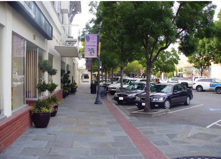
▼ Paving treatments can be used to accent the sidewalk by outlining trees or entire sidewalk zones
